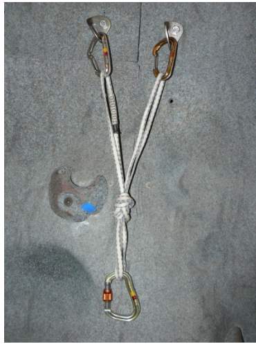
Figure 12 One sling with figure-8
