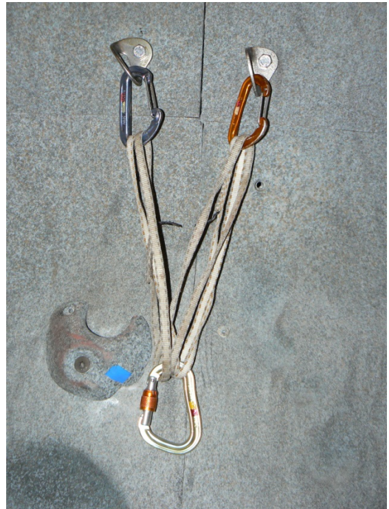
Figure 15 Sling X with two slings
