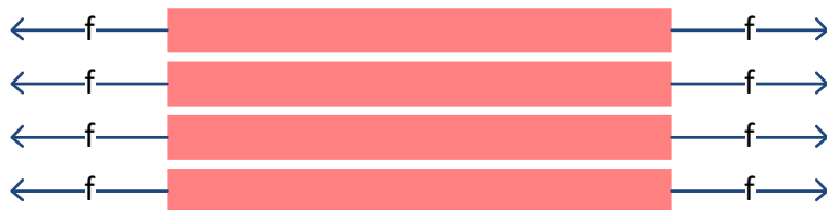
Figure 2 Force Distribution on a Straight Rope
